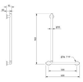
RIGHT-HAND ORIENTATION SHOWN, RAIL CAN ALSO BE SETUP FOR LEFT-HAND ORIENTATION.
